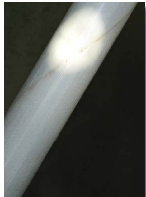
The above pole (showing white blistered area) continues to be cycled to 65% of original length at set of ten.
