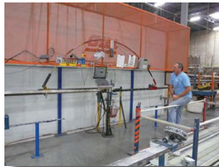
End load/flex testing of a vaulting pole.
