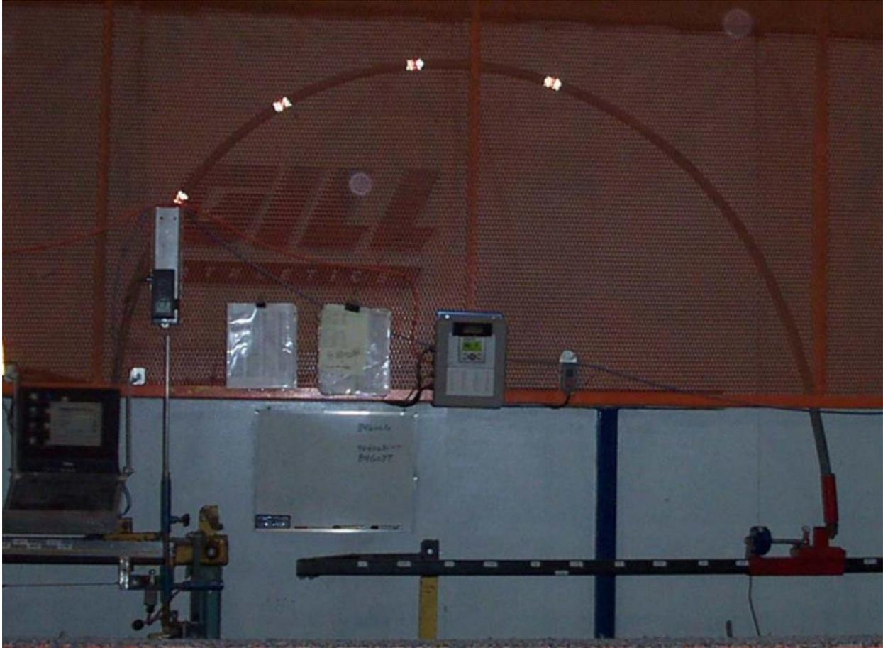
The load cell was attached at the right end in this picture – the carriage that the pole end was inserted into was on a roller bearing set up
